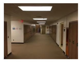
Photo 44. Sheet carpet flooring at 1st floor main corridor, 1968 addition, adjacent cafeteria. Carpet is worn and should be replaced with something more durable as this is a high traffic area. (Priority 0)
