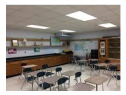
Photo 52. 2x2 Acoustical Ceiling Tile (ACT) system in the secondfloor classrooms, ceilings in good condition.
